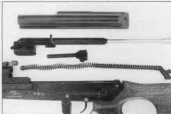
The VEPR .308 Carbine, fieldstripped — its Kalashnikov derivation is clear.
